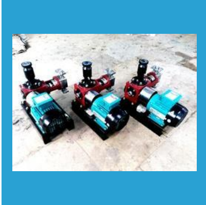
Chemical Dosing Pump
