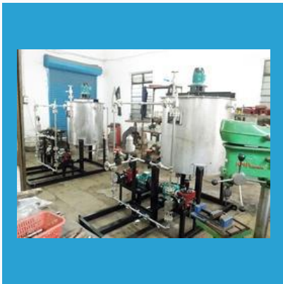
Skid Mounted Dosing System
